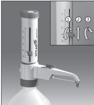
Variable: Loosen the volume selector thumb screw  $\frac{3}{4}$  turn (1), set the pointer to the desired volume (2) and then retighten the volume thumb screw (3).
